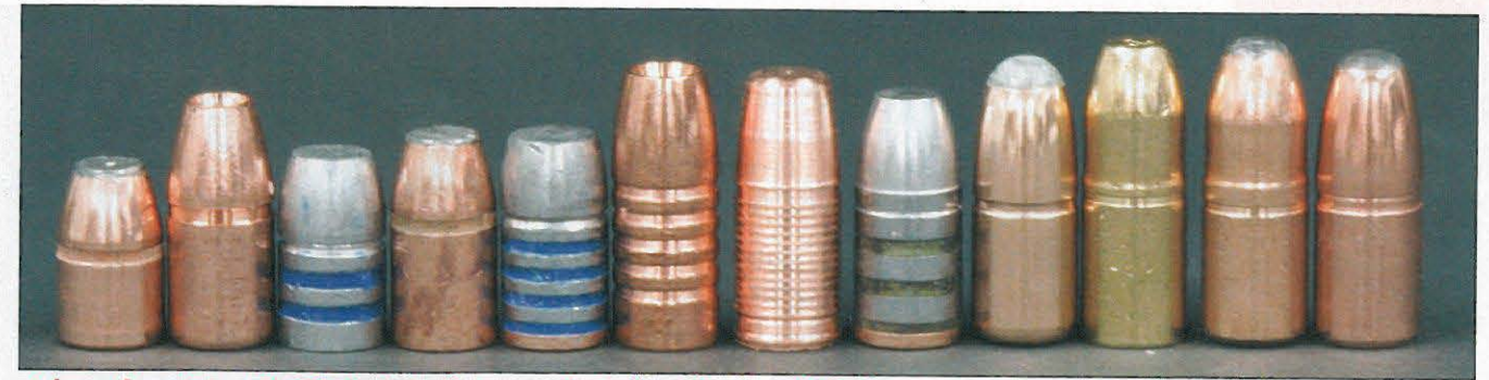
A broad variety of .475-inch bullets was tested and/or modified to produce optimum performance in heavy game. This lineup includes samples from 350-grain pistol bullets to 500-grain solids.
